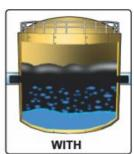
Our blend of additives will force any water contamination in the system to settle to the bottom of the sump so it can be easily drained off to protect the system.
